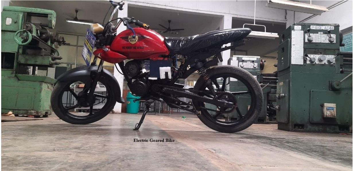
Electric Geared Bike – 750 Watt Capacity
