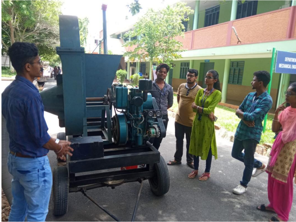
Vacuum Assisted Waste Collector for Campus Roads Cleaning Sponsored by NewGen IEDC
