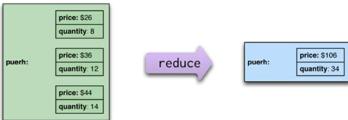
A reduce function takes several key-value pairs with the same key and aggregates them into one.
