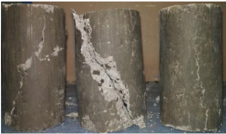
Fig. 3c: Tested UCS samples
